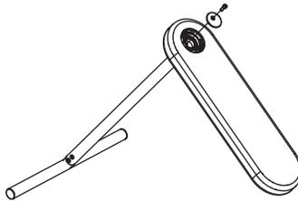
Step 3: Insert and lock in bar plate,
