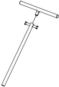
Step 2: Align bar plate with bar stem
